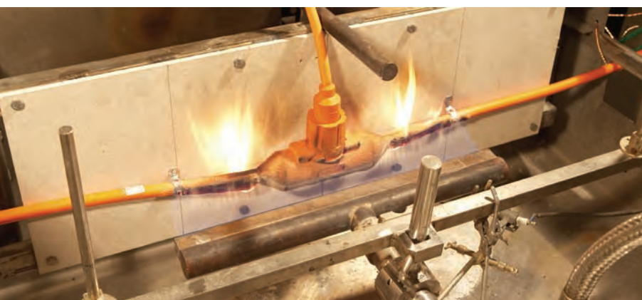
BS6387 Category Z - Resistance to fire with mechanical shock; 950°C for 15 minutes with 30 second hammer blows
